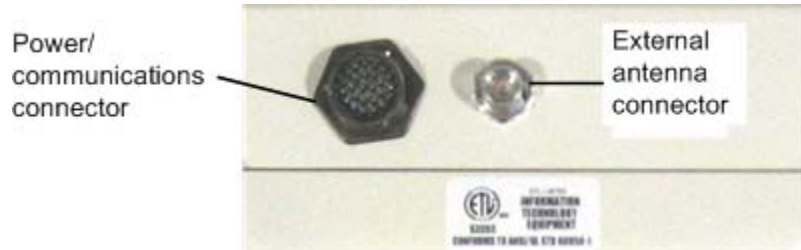
Figure 4-2 Back of Encompass 4 Reader Showing Antenna Connector
