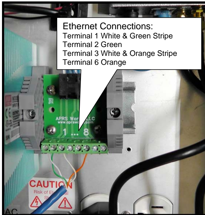
Figure 3 - Ethernet Terminal Block
