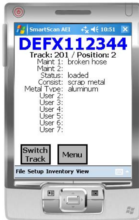
Figure 22 - Rail Vehicle Data Field Display
