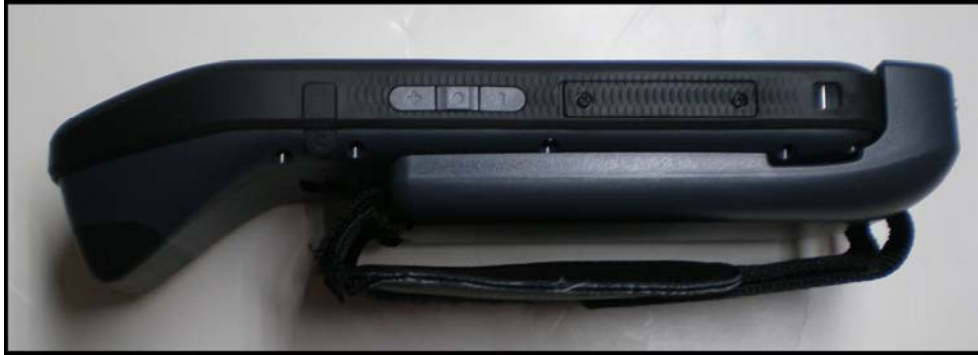
Figure 5 – External Battery Attached
